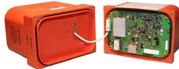
Figure 4: Battery Replacement for ELT Main Unit (Actual View)
