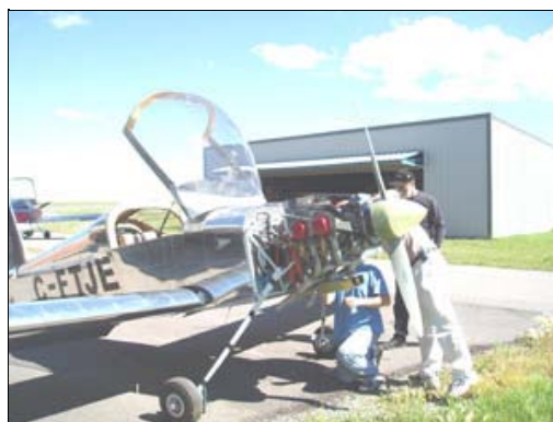
Prelubing engine before first start-up
