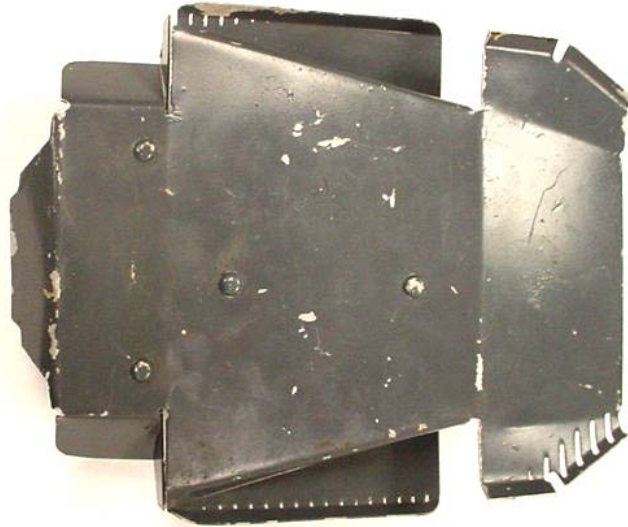
Figure 1: Lycoming baffle showing excessive signs of wear
